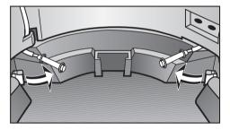
Unclip the water sensors and carefully bend them upwards.
